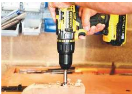
▲ A series of 35mm holes into beech with a Forstner was no problem
